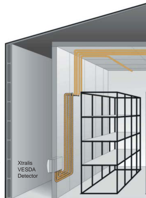
Figure 3. Xtralis VESDA detector located externally to the protected area
